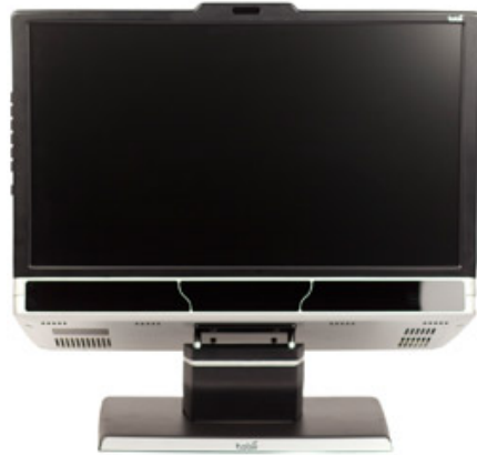
Figure 22: Tobii TX300 Eye-tracker. Screen size is 23 inches (557 mm wide) with 1920x1080 resolution. When a participant is seated 65 cm away from the screen, it will subtend about a 31 degree visual angle.
