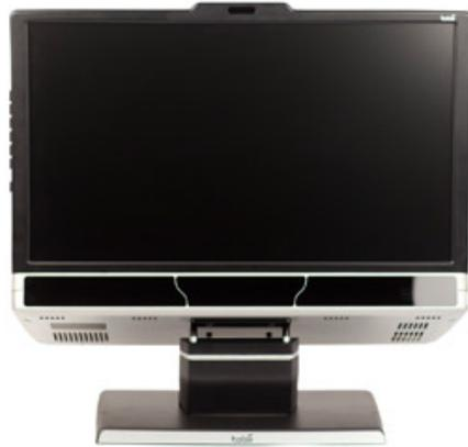
**Figure 3:** Tobii TX300 Eye-tracker. Screen size is 23 inches (557 mm wide) with 1920x1080 resolution. When a participant is seated 65 cm away from the screen, it will subtend about a 31 degree visual angle.
